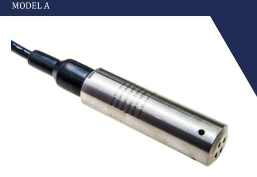
The 6549 MODBUS water level sensor is a pressure sensor-based instrument for measuring water depth in many applications. It has a cable with a vent tube for atmospheric pressure compensation. The 6549 water level sensor provides accurate long term measurements of water depths of 0m to 10m with an accuracy of 0.1% full scale. The sensor communicates via Modbus RTU RS485 protocol.
