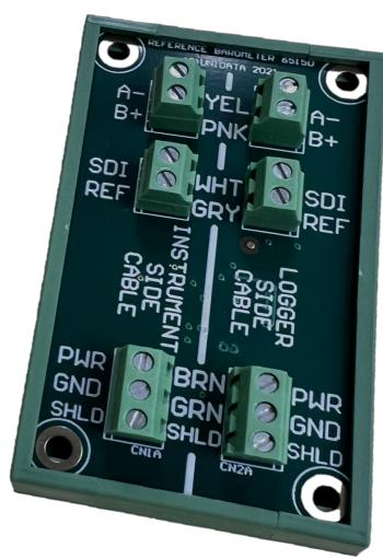
The Unidata 6515 is a barometric reference module which is used with the Starflow QSD SDI-12 instruments to correct the pressure sensor depth readings for atmospheric pressure variations.
