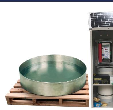
Unidata 6529-3 automatic evaporation monitoring system measures how much water evaporates from a Class A evaporation pan by measuring the water level in an adjoining stilling well. Use of stilling well reduces fluctuations in the pan's water level caused by wind.
