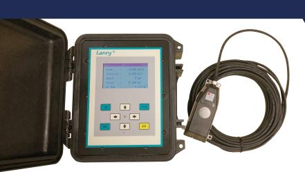
The DOF6000 series flowmeter consists of Flow Calculator and the Ultraflow 6537 Sensor, It is used to measure water velocity, depth, pressure temperature and conductivity of water flowing in rivers, streams, open channels and pipes.
