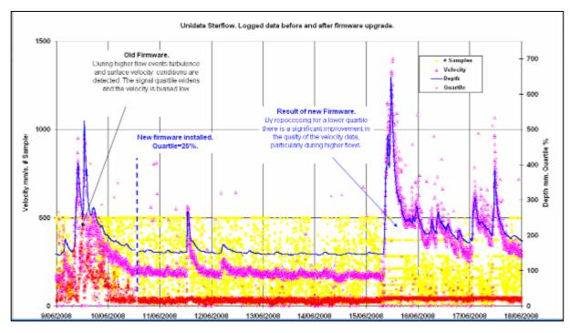
This compares with the continued poor quality of some velocity data logged by the control Starflow, shown on the following plot. The new firmware has significantly improved the quality of all, and particularly the higher velocity data.
