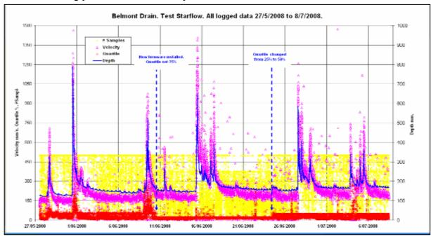
The following plot compares the depth / velocity relationship of data points with the old and new firmware to 24/6. Using the 25% quartile setting the new firmware generates some scattered and spurious high velocity data. This occurs when the algorithm is focussed too far onto the high velocity end of the signal spectrum.
