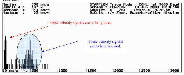
This "new firmware" solution was field-tested by Waterdata and a range of flow conditions were measured. This report summarises the results.
