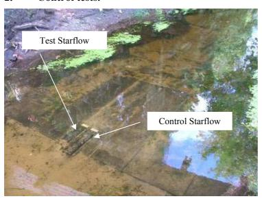
An existing Starflow that continuously logged the site depth and velocity was adjusted to include the signal Q and sample #, and used as the control throughout the tests.
