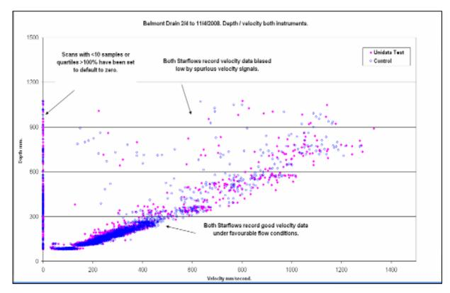
On 10/6/2008 the modified firmware was installed in the test Starflow. This was operated until 8/7/2008. A full range of flows were measured during this period.
