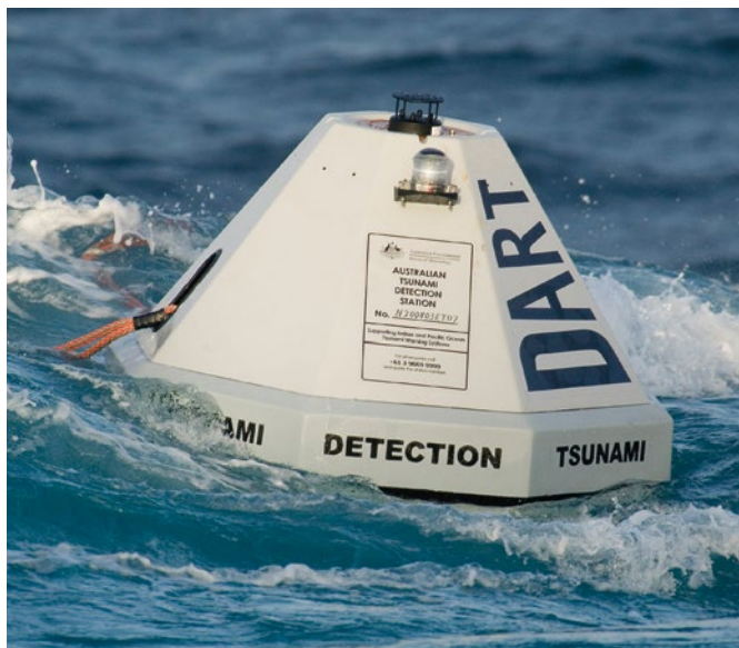
DART® real-time tsunami monitoring systems, developed by PMEL, are positioned at strategic locations throughout the ocean and play a critical role in tsunami forecasting.
