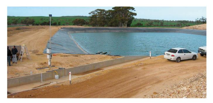
Surface water monitoring equipment measures surface water quality and quantity and transmits the information via cell phone or satellite to a central Neon Server where it can be analysed to make meaningful water management decisions.
