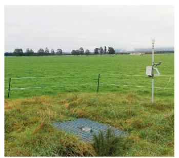
collection and transfer of data through its "plug and play" nature and soil moisture data is well presented on easy to understand graphs either on an iPad or Laptop. It is also easy to relocate the probe if needed.
