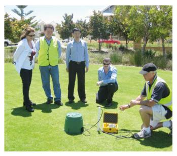
Modern soil moisture probes are reliable and affordable. Telemetry options, like mobile phone or satellite network modems are becoming more and more affordable as well. Moving data from the field to the website as well as access to this data through either, mobile web browsers or specialised mobile apps, makes it easy for turf manager and irrigators to check soil moisture readings whenever they need.
