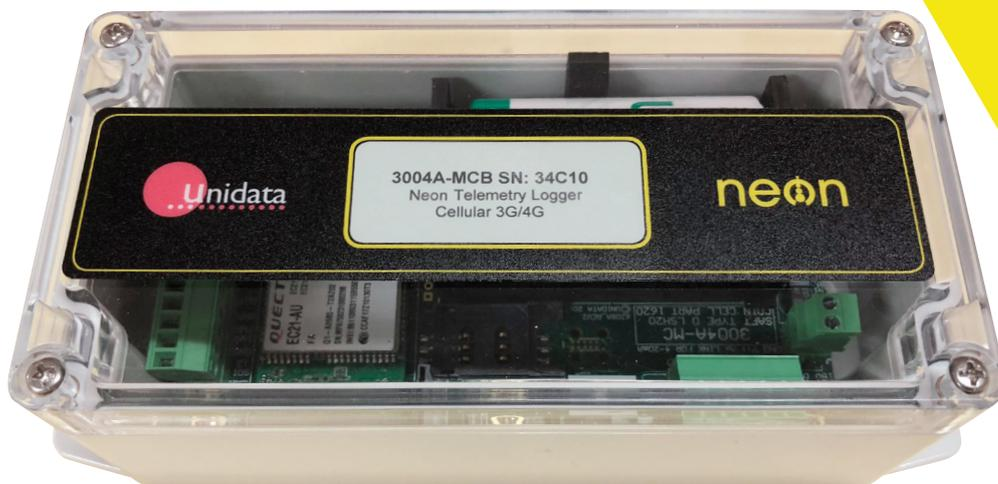
The 3004MC Neon Metering Logger Cellular is a Neon Metering Logger in the 3004M range which has a smaller form factor than the standard metal enclosure 3004. It is housed in a polycarbonate case. It utilises the Cellular phone networks as its method of sending sensor data from the field to the Neon Server.
