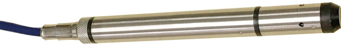
The 6542 hydrostatic water depth and temperature probe is a pressure sensor based instrument for measuring water depth in many applications. It has a cable with a vent tube for atmospheric pressure compensation. The 6542 Hydrostatic water depth and temperature probes provide accurate long term measurements of water depths of 3m to 50m in standard ranges, with an accuracy of 0.05% full scale. Sensor communicates via SDI-12 v1.3 or Modbus RTU RS485 protocol.
