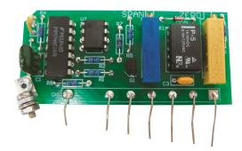
Isolated interface input module model 6141A for use with Starlogger and model 7121A for use with Prologger provides isolation for transducers which cannot be directly connected to a datalogger e.g. current loop transducers.
