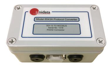
The 6543 Babelstar Protocol Converter converts Modbus to SDI-12 requests OR converts HSIO data into Modbus data. SDI-12 is a standard protocol, defined by the USGS, which defines how a sensor must communicate with a datalogger via an SDI 12 bus. HSIO is a Unidata proprietary protocol for connection of Unidata dataloggers to displays and instruments.
