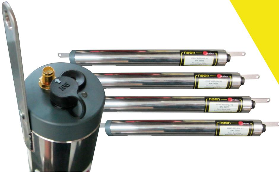
The 2024 Neon Remote Terminal NRT is small self-contained data logger/rtu in a tubular stainless steel housing which connects to downhole sensors in bore holes, collects readings from those sensors and transmits the collected data to a central Neon server. The model number suffix indicates data transmission via a cellular 2G/3G network or via a cellular 4G/LTE network. The 2024 terminal is designed as a telemetry system for bore holes with diameters of 50mm or greater.
