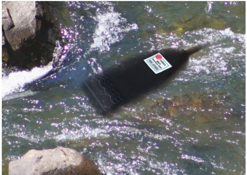
an ultrasonic velocity sensor, vent tube inclusion for pressure sensor compensation becomes redundant, making 6527 an easier instrument to deploy. On top of that, 6527 is a completely sealed unit, so there is no possibility of water ingress into the electronics inside the instrument or need to use drying desiccant tube.
