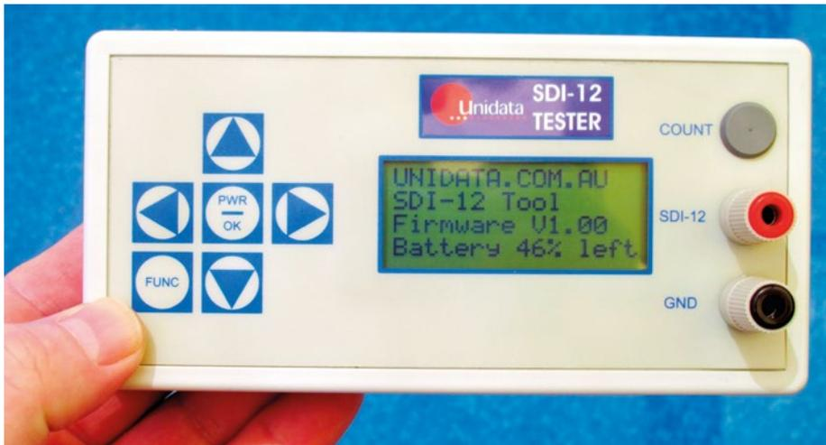
The tester is battery powered and has the ability to perform the functions, Monitor bus, Query address, acknowledge active, change address, send identification, start measurement, send data, send extended command and cyclical measure & send data.
