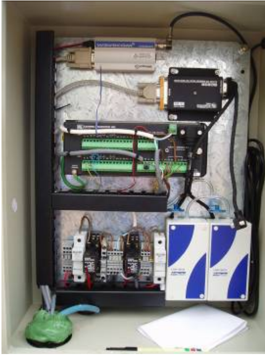
Figure 7 Example of logger enclosure setup from Myuna station.
