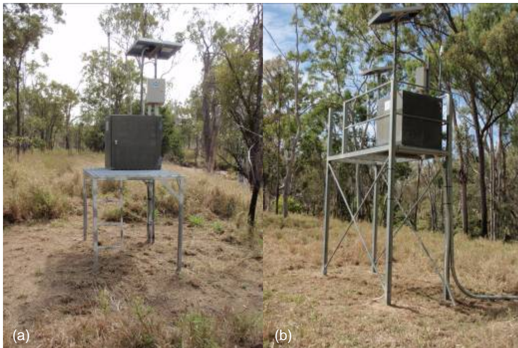
Figure 1 Examples of small platform design (a) at Thornton Creek and large platform (b) at Keelbottom Creek both located on the Department of Defence Townsville Field Training Area.
