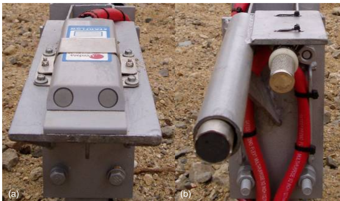
Figure 4 Starflow velocity probe mount (a) and turbidity probe mount (b).
