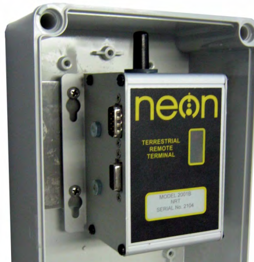
NRT Example which is secured within a Weatherproof Enclosure
