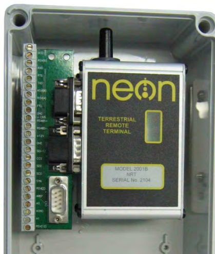
An NRT installed with FTS connected
