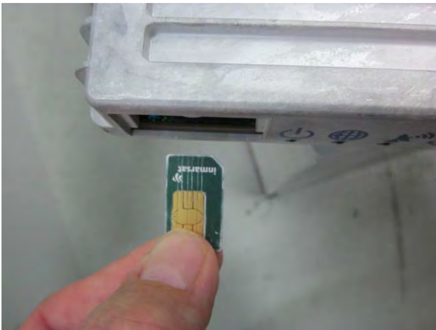
Insert the SIM card with the notch orientated as above.
