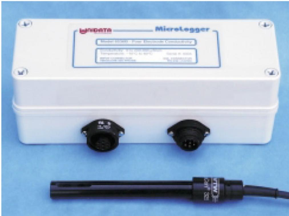
The instrument includes an integrated Starlog-compatible MicroLogger, providing all the standard features found in Starlog such as SDI-12 communications, intelligent battery supervision, a modem interface, and all the programmability found in Starlog Data Loggers.
