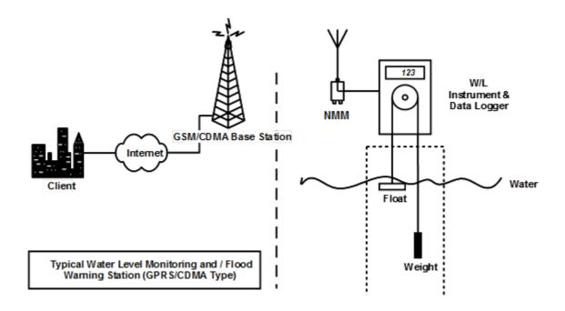
The figure above is an example of a Neon installation showing an NRT connected to a Water Level Instrument. Every day the NRT will send a "packet" of information containing the data in raw format via GSM / 3G to the Neon server. The Neon server extracts the raw data from the packet. The data is then stored on a secure server until the client accesses the data using a standard Web Browser.
