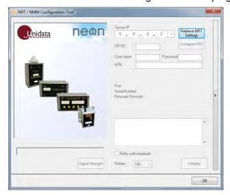
Press the 'Signal Strength' button. After a short delay (10 seconds or so), the RSSI signal strength will be displayed. RSSI must be 16 or higher. If it is 99 then there is no connection to the cellular network.
